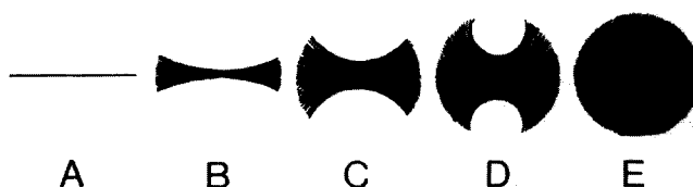
Figure 6 Evolution of spherulitic growth ranging from a folded-chain single crystal (A) to a fully developed spherulite (E)
